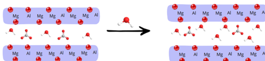
Figure 6. Mechanism of water molecule adsorption by Mg/Al hydrotalcite [22]
