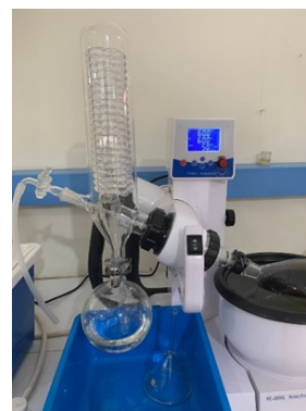
Figure 2. Evaporation of solvents using a rotary evaporator
