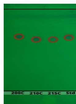
Figure 1. TLC chromatogram of caffeine in coffee samples under UV light (254 nm)
