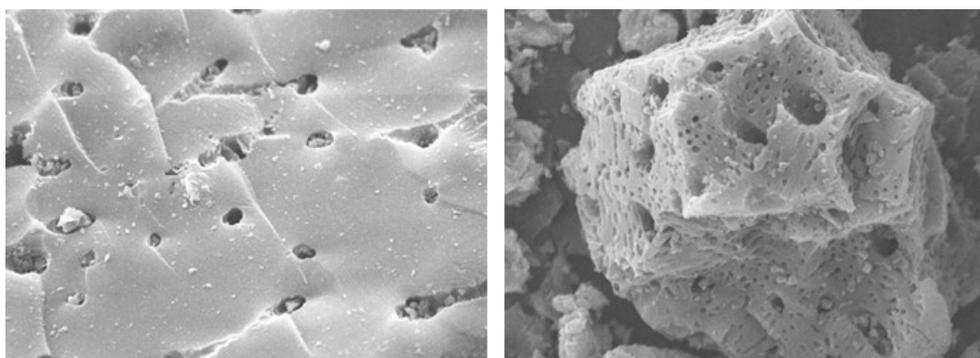
**Figure 3.** SEM micrograph of a) carbon non activation and b) activated carbon (KAF)
