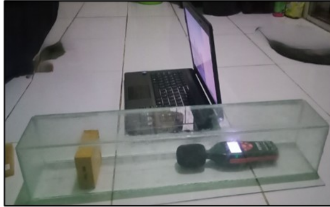
Figure 2. Method of taking sound intensity data at different frequencies
